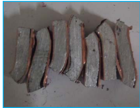
Delaminated after cutting (①、⑤) 套管法锯切后开裂照片
