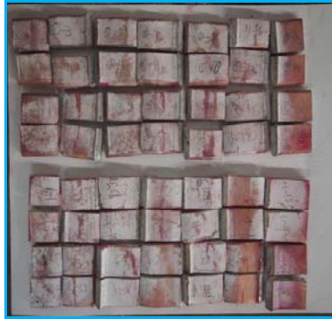
Bonded well After Cutting (1、5) 水平连铸法锯切后试样照片
