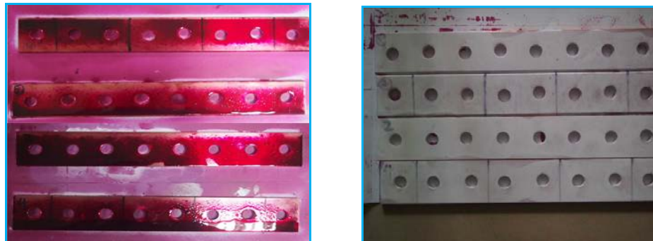
Liquid Penetrant Examination 着色渗透探伤检验
